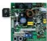
SPA30 spare control unit, only card, for SP6100
