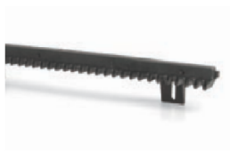
r0A6 M4 25x20x1000 mm slotted nylon rack with metal insert for gates weighing up to 500Kg
