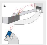
OXIT, OX2T AND OX4T RECEIVERS CAN BE USED AS SIGNAL REPEATERS.
